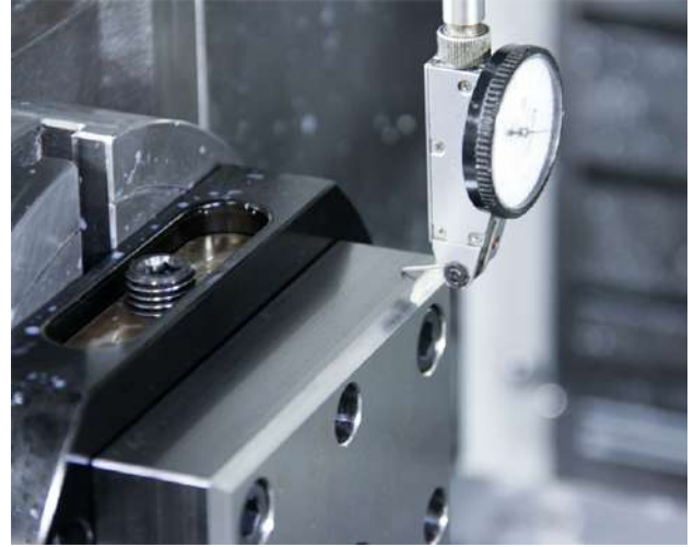
Precision milled sides allow for indication of center line.
